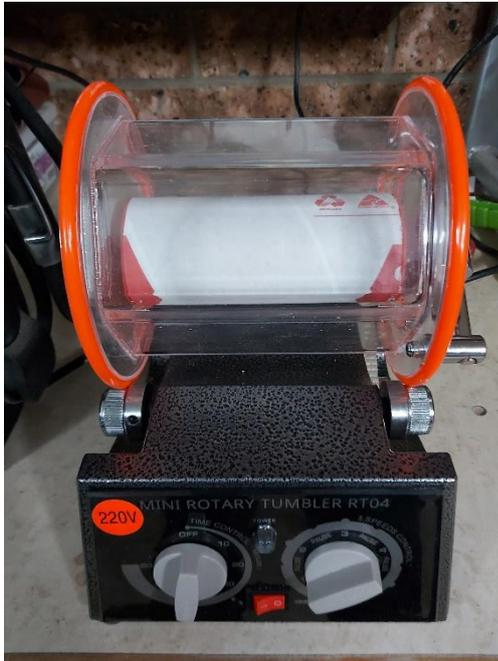
germinate difficult species. Rather than damage the polycarbonate cylinder, I cut down a poster cylinder I purchased at the post office. The cylinder is 60mm in diameter. Into this I inserted a piece of 80 grit sandpaper, so that the seed would be continuously in contact with the sandpaper as the cylinder turned. The end caps provide a tight fit so even small seed would not escape.
